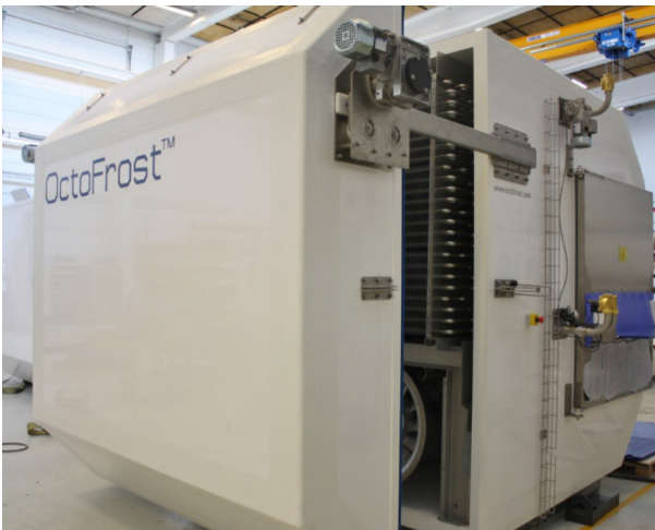
Figure 5. An IQF unit with a mobile lateral door
