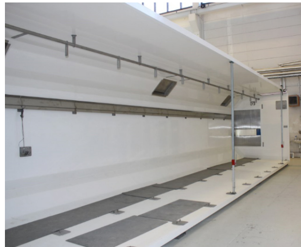
Figure 6. An IQF unit with a mono-block casing
